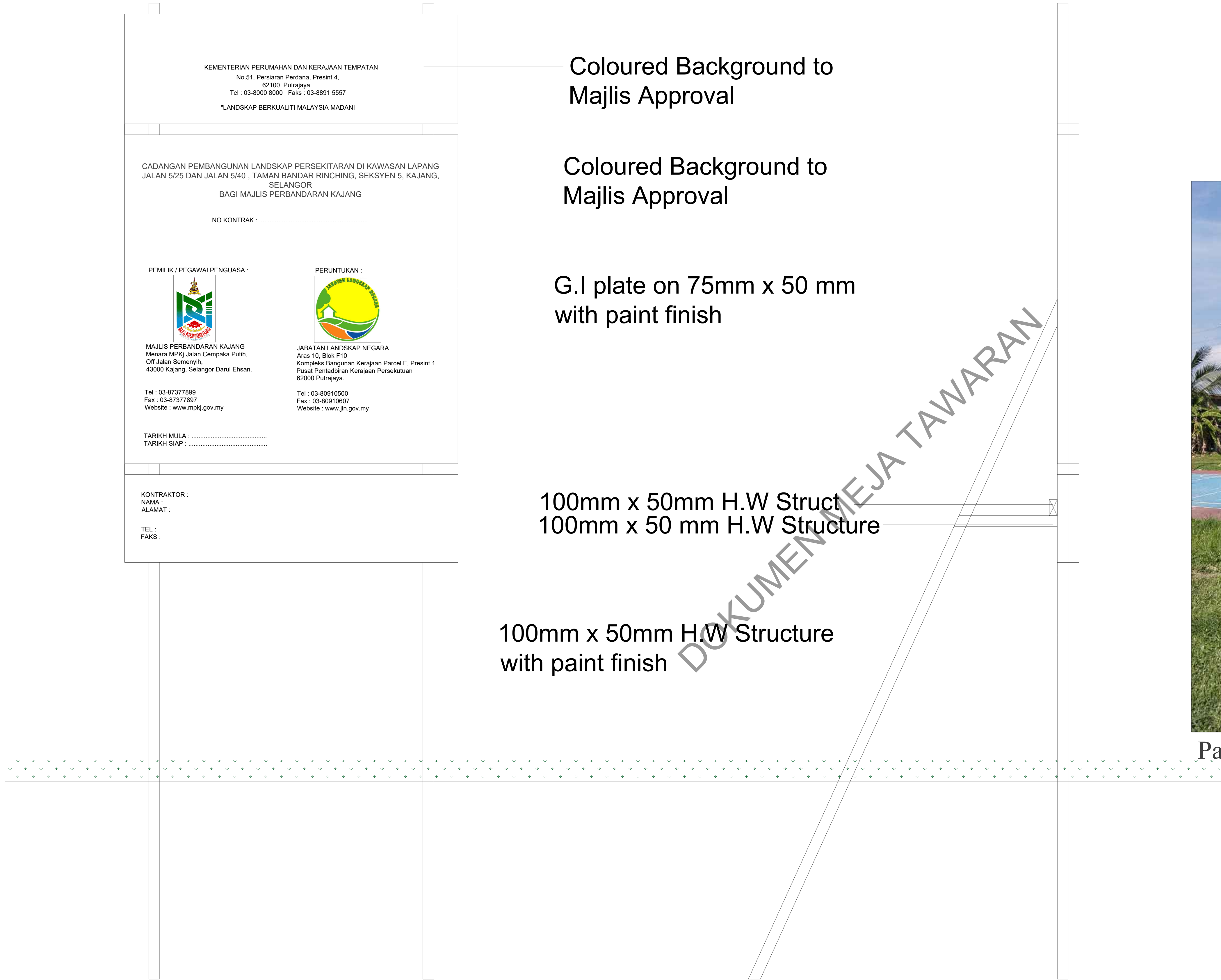
SECTION PAPAN TANDA PROJEK SKALA 1:10
